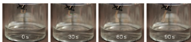
Figure 11. Demonstration of chemo-responsive shape-memory behavior. A 2b \cdot \text{Eu}(\text{NTf}_2)_3 film was fixed into a bent shape using UV light and suspended above methanol in a sealed container. Methanol affects the stability of the metal–ligand complexes, which results in decreased phase separation that leads to recovery of the permanent shape.
